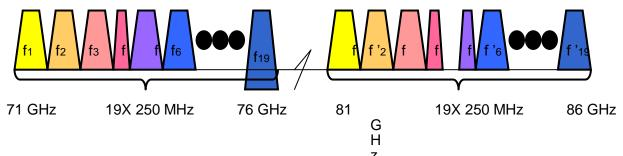
Based on recommendation from ITU-R F.2006, the proposal of channel arrangements for Channel Spacing of 250MHz and 500MHz is basically same
